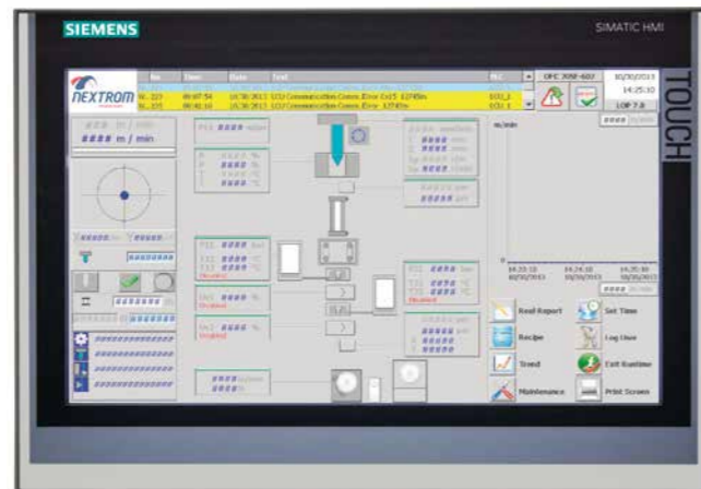
Line control screen
