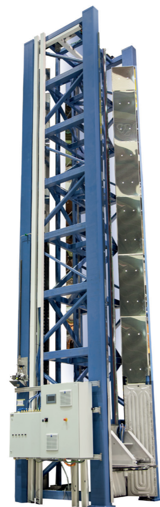
Tall preform feeding unit for up to 230 mm preforms
